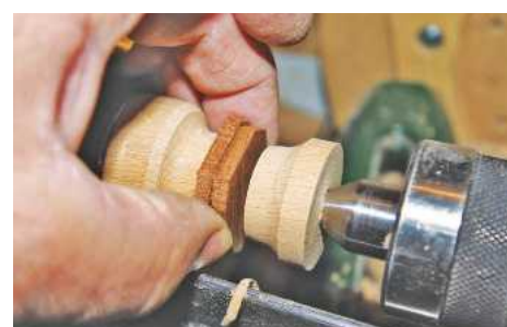
▲ Pic.6 Pinch two pieces of mahogany between the platens and turn down by a couple of millimetres
